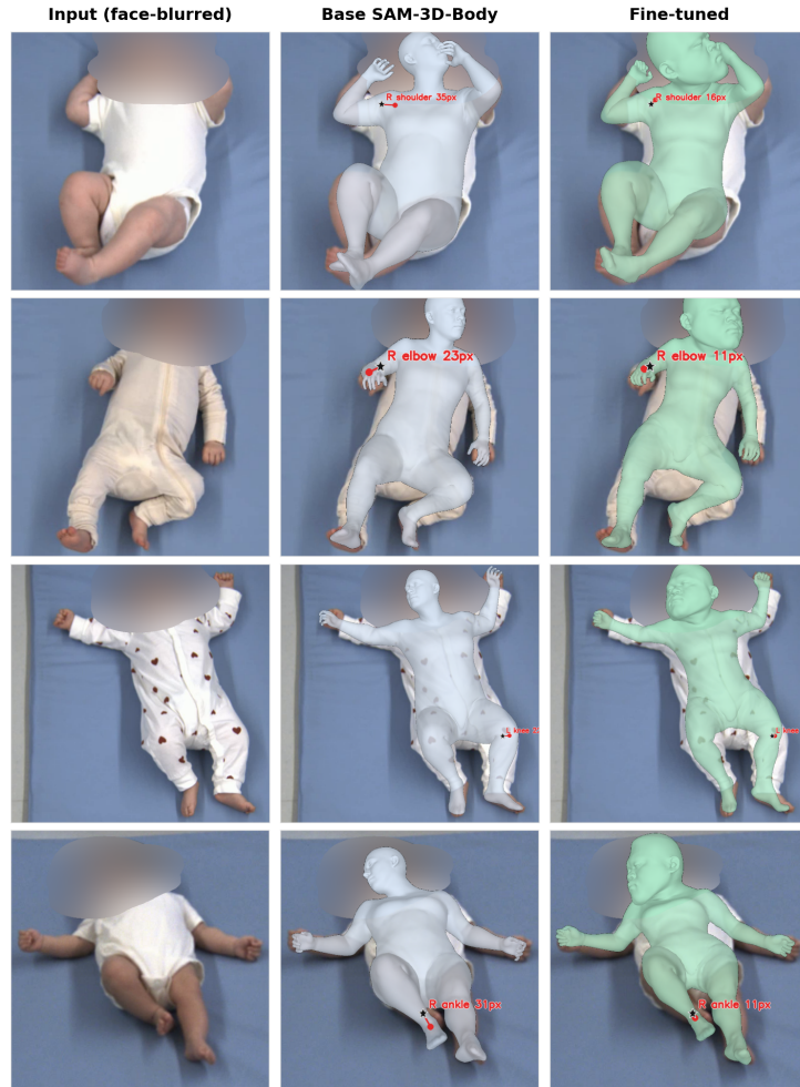
Fig. 2: Qualitative comparison on four held-out infants (rows), through the capture rig’s shared elevated camera. Columns: face-blurred input; base SAM-3D-Body mesh; fine-tuned mesh. For each row we highlight the major limb joint where fine-tuning most reduced the 2D distance to the Sapiens teacher keypoint for that frame and camera; a black star marks the Sapiens target, and the line and label on each mesh column give that model’s pixel distance to it (fine-tuned consistently closer). Targets are the Sapiens-Goliath 2D keypoints, computed as in our prior study.
