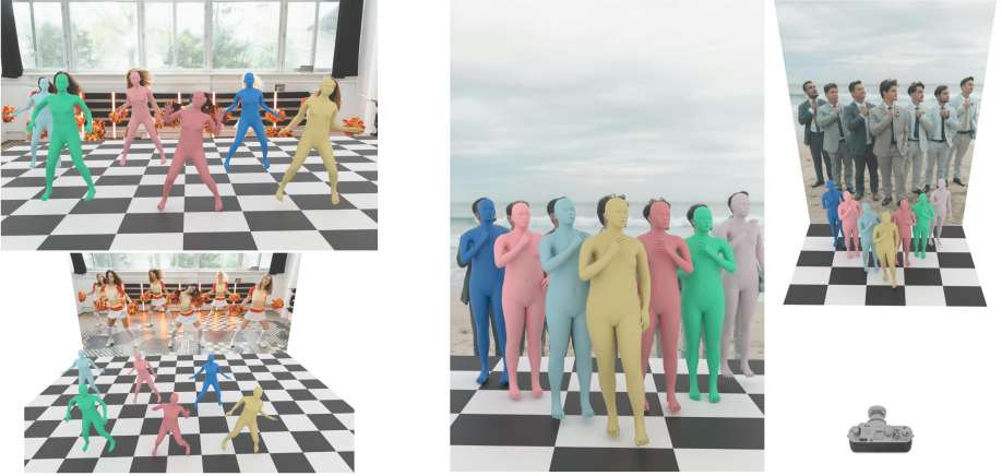
Fig. 1: Multi-HMR 2 detects humans and recovers their 3D meshes, placed in the scene, along with camera parameters. It also outputs per-human features that allow online tracking in videos, despite being trained only on still images.
